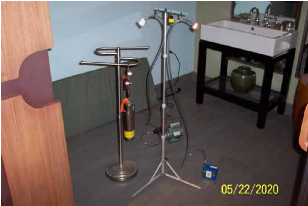
Photo No. 7 View of background air sample being collected on the second floor of the Sunlighten Saunas building.
